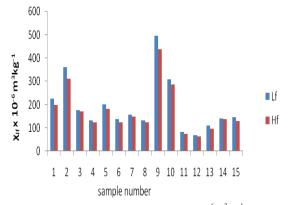
Figure 6: Magnetic susceptibility values (  $x \ 10^{-6} \ m^3 kg^{-1}$ ) for JCOE samples both at high and low frequency.
