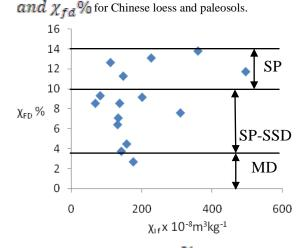
**Figure 13.** A schematic  $\chi_{lf} - \chi_{fd}$ % scattering diagram showing typical positions of samples from JCOE.
