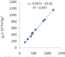
**Figure 8:** Relation between low frequency and high frequency susceptibility for Jalingo motor park.
