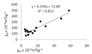
**Figure 10:** Linear regression between  $\chi_{fd}$  and  $\chi_{Lf}$  for JCOE samples.
