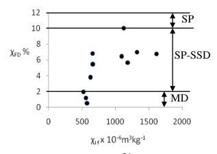
**Figure 14**: A schematic  $\chi_{lf} - \chi_{fd}$ % scattering diagram showing typical positions of samples from JMM.
