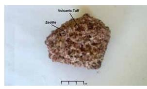
Figure 5: Reddish zeolitic tuff sample from HV.
