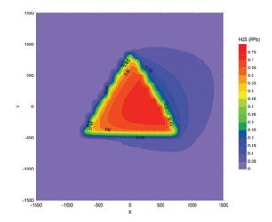
**Figure 4**. Contour plot for annual  $H_2S$  (ppb) in the vicinity of ASWWTP which is assumed to be at the center of the map at coordinates (0, 0)
