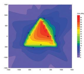
**Figure 6**. Contour plot for 24-hours methane (ppb) in the vicinity of ASWWTP which is assumed to be at the center of the map at coordinates (0, 0)
