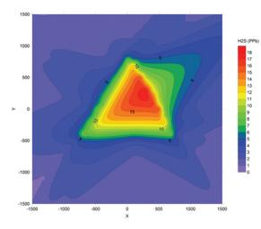
Figure 2. Contour plot for predict one-hour  $H_2S$  (ppb) in the vicinity of ASWWTP which is assumed to be at the center of the map at coordinates (0, 0)
