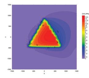
**Figure 7**. Contour plot for annual methane (ppb) in the vicinity of ASWWTP which is assumed to be at the center of the map at coordinates (0, 0)
