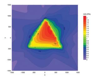
Figure 3. Contour plot for predict 24-hours  $H_2S$  (ppb) in the vicinity of ASWWTP which is assumed to be at the center of the map at coordinates (0, 0)
