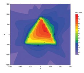
**Figure 9**. Contour plot for 24-hours ammonia (ppb) in the vicinity of ASWWTP which is assumed to be at the center of the map at coordinates (0, 0)
