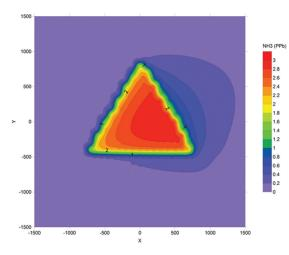
Figure 10. Contour plot for annual ammonia (ppb) in the vicinity of ASWWTP which is assumed to be at the center of the map at coordinates (0, 0)
