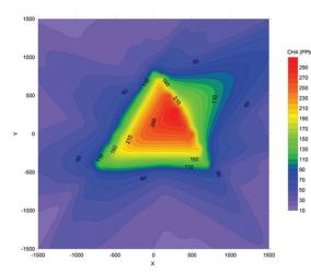
**Figure 5**. Contour plot for one-hour methane (ppb) in the vicinity of ASWWTP which is assumed to be at the center of the map at coordinates (0, 0)
