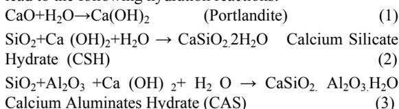
The compressive strength results of ash glass sand mortars have shown that the compressive strength at 7 days is low when compared with the 28 days results, this is related to the longer curing time which gave the opportunity to the ash alkalis to react with the silica to form extra cementitious matrix.
