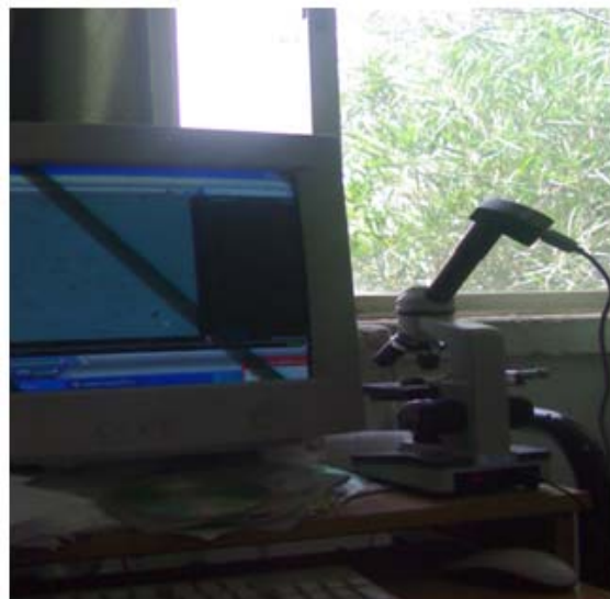
Fig 2. Digital microscope with USB camera.
