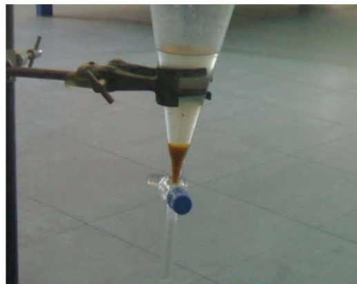
Fig 3 Extraction of Beta Carotene.
