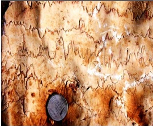
**Figure 7.** Vertical peak stylolite, sharp peak with high amplitudes, the shortening ratio in this sample is 11% as a result of stylolitization (Shtafina area).
