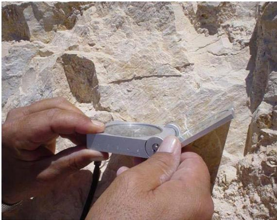
**Figure 3:** Slickenlines show a normal-dextral movement of a fault plane.
