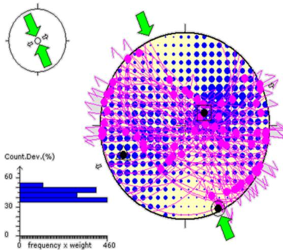
**Figure 10:** Principal stress axes determination by using the TENSOR program; outward ENE arrows indicate tension ( $\sigma_3$ ) and inward NNW arrows indicate compression ( $\sigma_1$ ), while  $\sigma_2$  is vertical.
