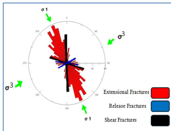
**Figure 9:** Strike orientation of 740 fracture planes and the generalized direction of maximum principal stress axis ( $\sigma_1$ ) parallel to extensional fractures and minimum principal stress axis ( $\sigma_3$ ) parallel to release fractures.
