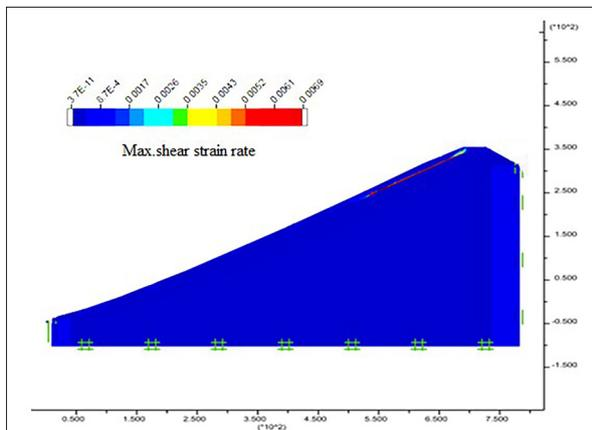
Figure 17. Failure mechanism 1 (Short term limit analysis).
