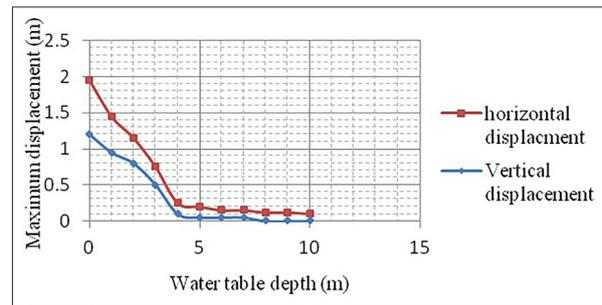
**Figure 13.** Curves of variation of horizontal displacements and vertical displacements as a function of the water table depth.
