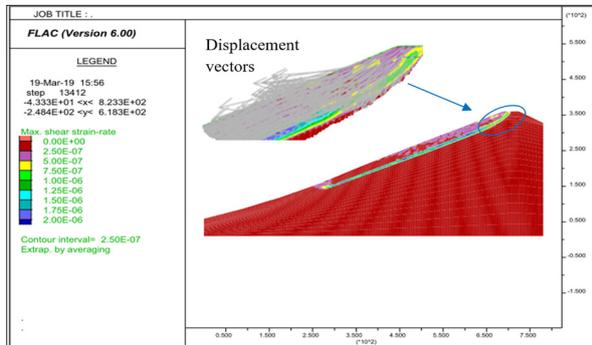
Figure 20. Failure mechanism 3 (Moderate piezometric height).
