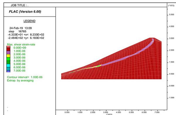
Figure 22. Failure mechanism 4 (Average drainage level and low cohesion)
