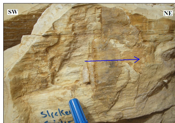
Figure 8. Slickenlines with calcite steps as a sense of movement indicator of sinistral strike-slip fault, in which the missing plane moved in the direction of the blue arrow.
