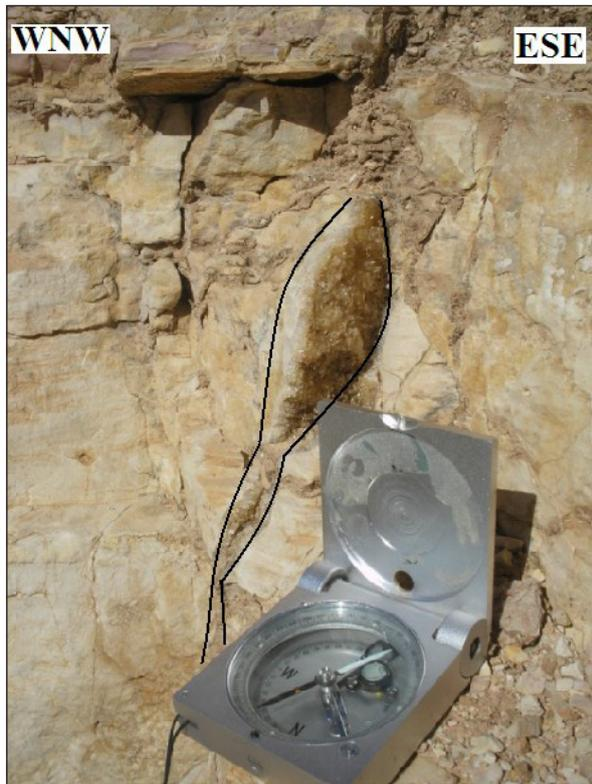
Figure 12. Karstified throughgoing fracture filled with calcite.
