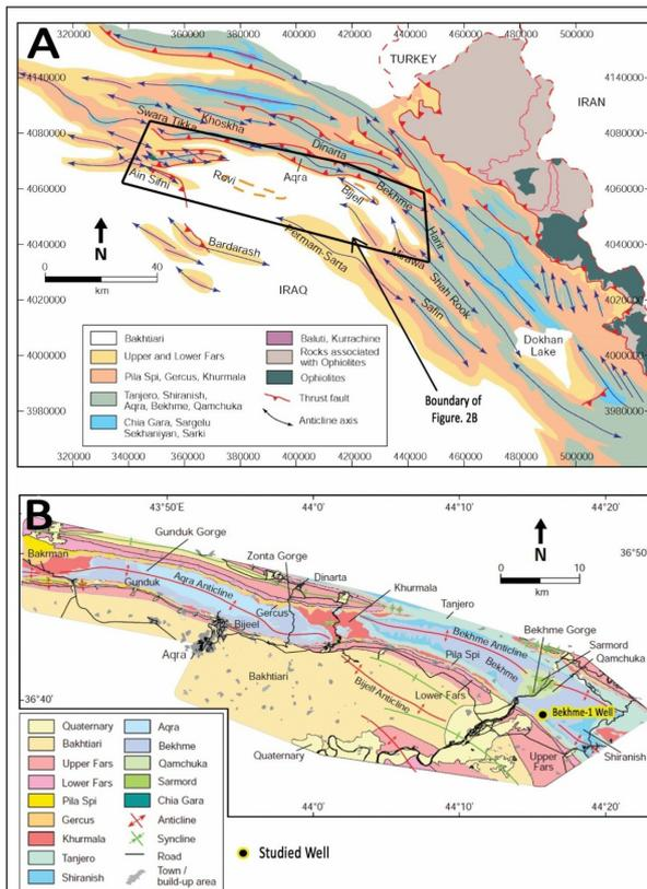
**Figure 2.** A. Schematic geologic map of Northern part of Iraq showing generalized geologic formations and trends of anticline axes (after Csontos et al., 2012). B. Detailed geological map of the area with an indication of the studied well, the map showing the two main anticlines to the north that correspond to the Aqra (western) and the Bekhme (eastern) (after Csontos et al., 2012).
