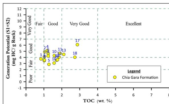
**Figure 6.** Cross plot of TOC wt.% versus Generation Potential (GP) shows the fair to good potentiality (Alaug et al., 2014).
