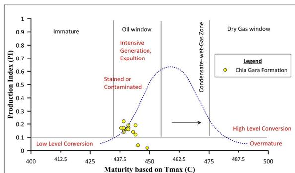
**Figure 11.**  $T_{max}$  vs. Production Index (PI) diagram of the Chia Gara Formation (adapted from Atta-Peters et al., 2015).
