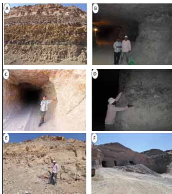
Figure 3. Field photographs showing Aswan kaolinitic clays; A) varicolored kaolinitic clays at Wadi Abu Aggag; B) room and pillar method for raw material extraction; C) the passage for underground mining; D) pale to dark grey bed with plant remains; E) sandstone cap-rock of the upper part of the Timsah Formation at Wadi Abu Subeira; and F) operating interface at Wadi Abu Subeira.
