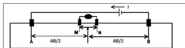
Figure 2. Schlumberger Configurations Array
