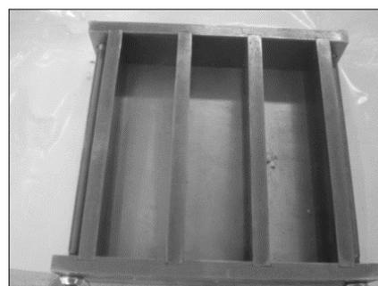
a. Compressive and flexural mold
