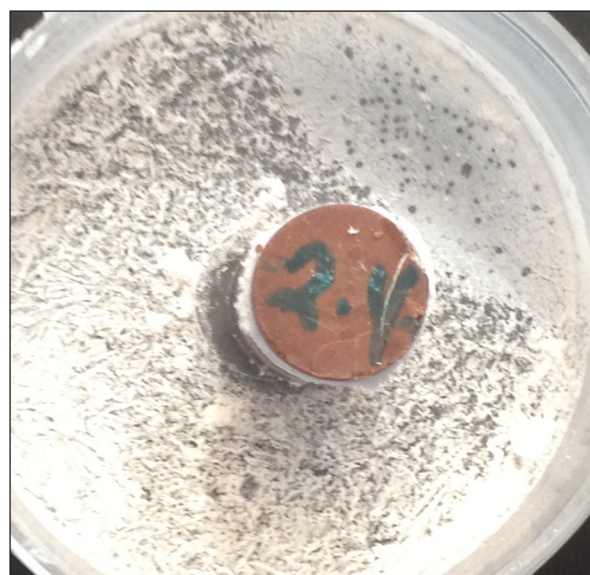
Figure 6. Extent of alkali leaching (efflorescence) observed in the samples.
