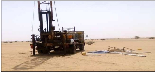
Figure 2. General view of the study area condition showing the used drilling rig machine for the SPT test and soil sampling
