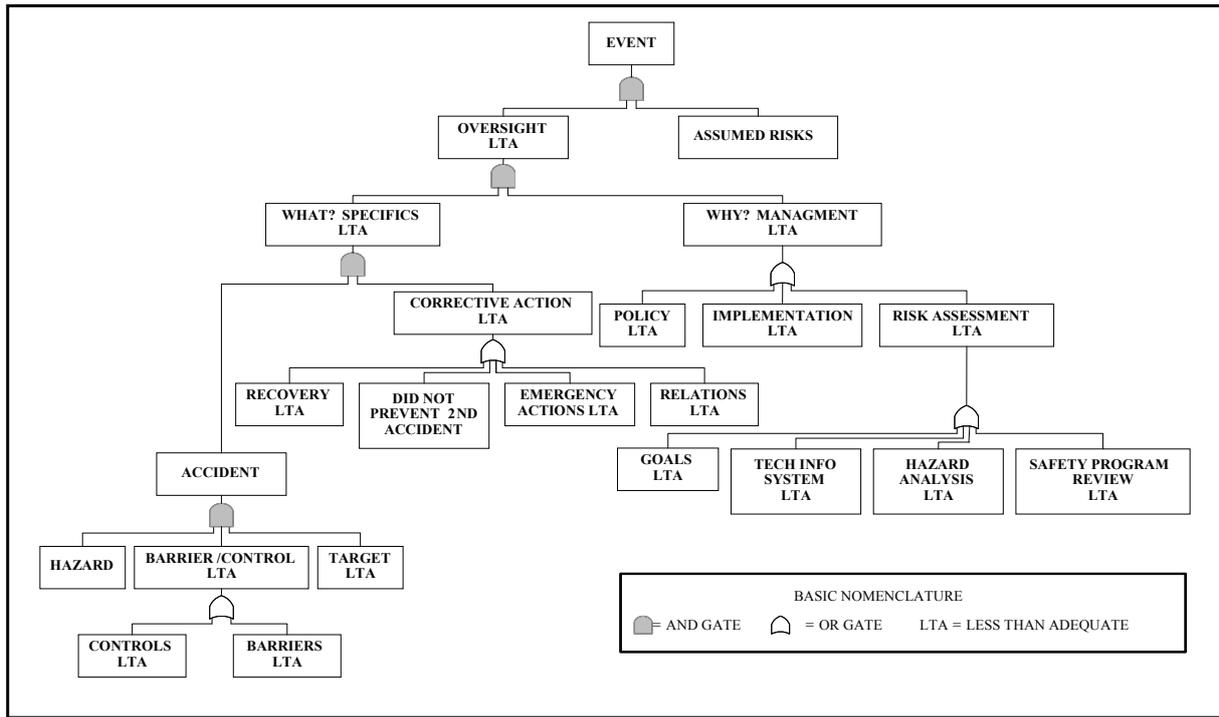
Figure 3: Overview of the Basic Structure of MORT (Adapted from NRI-1, 2002).
