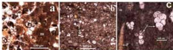
**Figure 7:** MFT1 Phosphatic foraminiferal wackestone. a) represents the lowest 4 m of the section Fig. 2, b) from the 4.5 m marly limestone, 10 m from the base, c) From the 60 cm limestone horizon mid section. p, phosphate particles; f, foraminiferal test; m, matrix. Plane polarized light (PPL).
