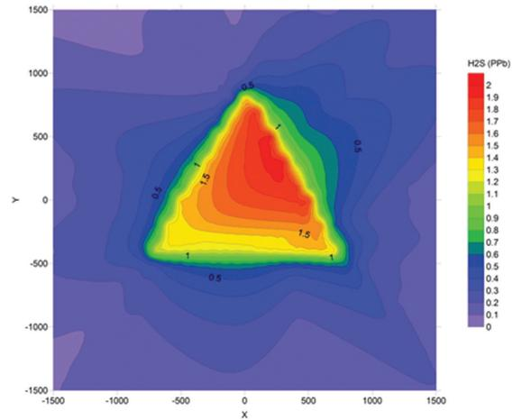
**Figure 3.** Contour plot for predict 24-hours H<sub>2</sub>S (ppb) in the vicinity of ASWWTP which is assumed to be at the center of the map at coordinates (0, 0)
