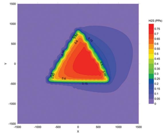
**Figure 4.** Contour plot for annual H<sub>2</sub>S (ppb) in the vicinity of ASWWTP which is assumed to be at the center of the map at coordinates (0, 0)
