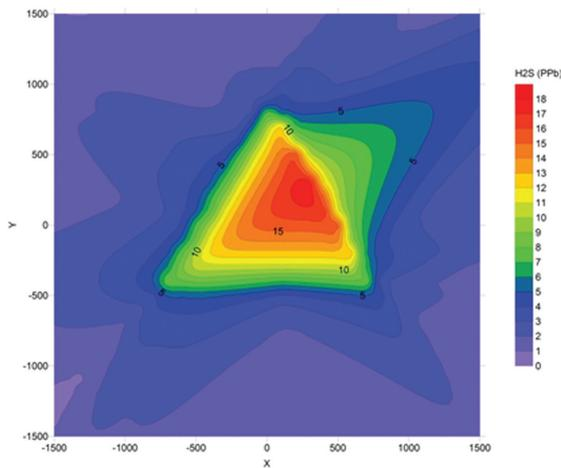
**Figure 2.** Contour plot for predict one-hour H<sub>2</sub>S (ppb) in the vicinity of ASWWTP which is assumed to be at the center of the map at coordinates (0, 0)
