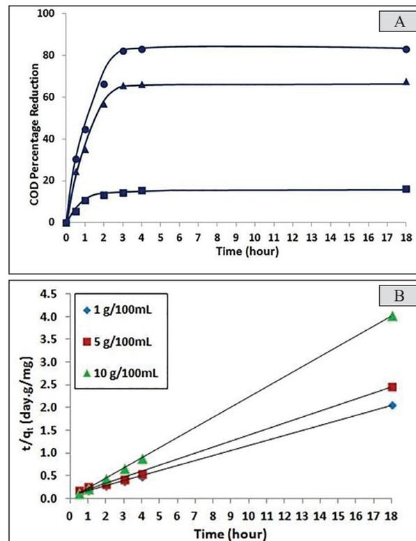
**Figure 2.** (A) Percentage COD removal as a function of time for different particle dosages (squares for 1 g/100 mL, triangles for 5 g/100 mL and circles for 10 g/100 mL), all at pH=6, 22°C and a stirring rate= 250 rpm. (B) Second order kinetic model for the adsorption of organic molecules onto stone cutting particles for different particle dosages.
