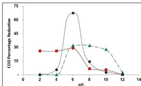
**Figure 5.** Equilibrium removal efficiency as a function of solution pH using a particle dosage of 5 g/100 mL, at a temperature of 22°C and a stirring rate of 70 rpm (squares for soil, triangles for marlstone, and circles for stone cutting).
