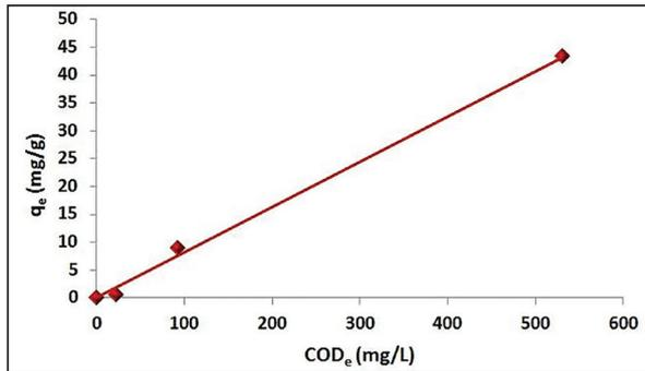
**Figure 6.** Adsorption equilibrium isotherm as a plot of equilibrium concentration in the solution versus surface concentration, for equilibrium experiments with a particle dosage of 10 g/100 mL, pH=6, and at a temperature of 22°C.
