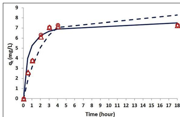
**Figure 1.** Experimental kinetic curve of  $q_t$  (organics load on the adsorbent) and model curves using pseudo first order rate equation (dashed line) and second order (solid line), for adsorption experiments using stone cutting solid waste with a particle dosage of 5 g/100 mL at a temperature of 22°C, pH= 6 and stirring rate= 250 rpm.
