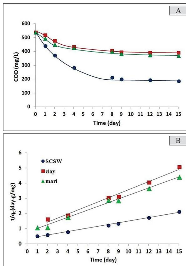
**Figure 4.** (A) Adsorption kinetics (COD versus time) for static conditions (no stirring) with a particle dosage of 5 g/100 mL of adsorbent, at a temperature of 22°C and pH= 6 (squares for soil, triangles for marlstone and circles for stone cutting). (B) Second order kinetic model for the adsorption of organic molecules onto various mineral adsorbents for stagnant particles
