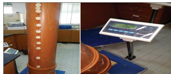
Figure 3. Column of soil and the digital balance.
