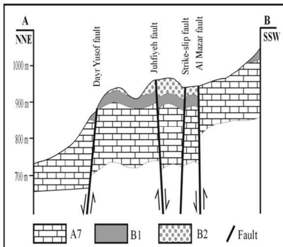
Figure 3: N-S cross section in the area (based on boreholes data). The location is shown on the map of Figure 2.
