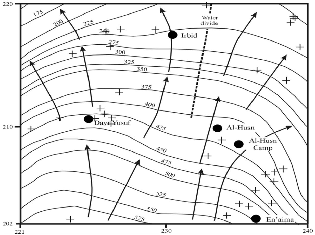
Figure 5: Groundwater flow in Irbid area. Contour lines represent the groundwater level. Crosses represent boreholes locations.
