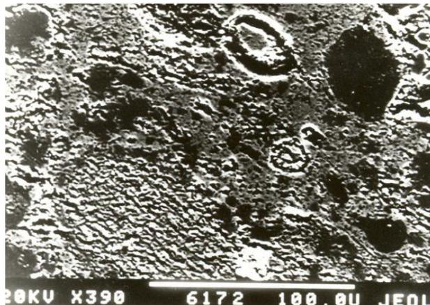
Fig. (9): Apatite (microcrystalline to amorphous) occurs as dark envelopes surrounding light cores of phosphate particles (pellets)
