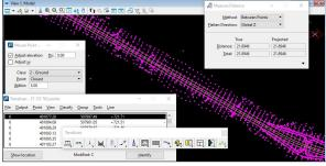
Figure 3. Cross section points measured using Total station every 25m along the Road.
