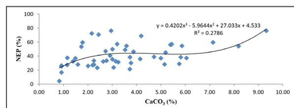
Figure 4. Mean non-erodible soil particles (NEP) versus CaCO<sub>3</sub> content
