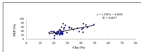
Figure 1. Mean non-erodible soil particles (NEP) versus clay content
