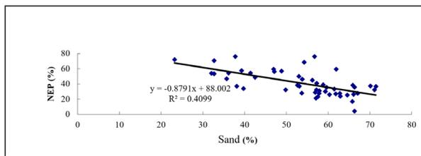
Figure 5. Mean non-erodible soil particles (NEP) versus sand content
