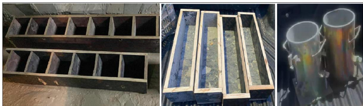
(a) Molds of Concrete Compressive Strength
