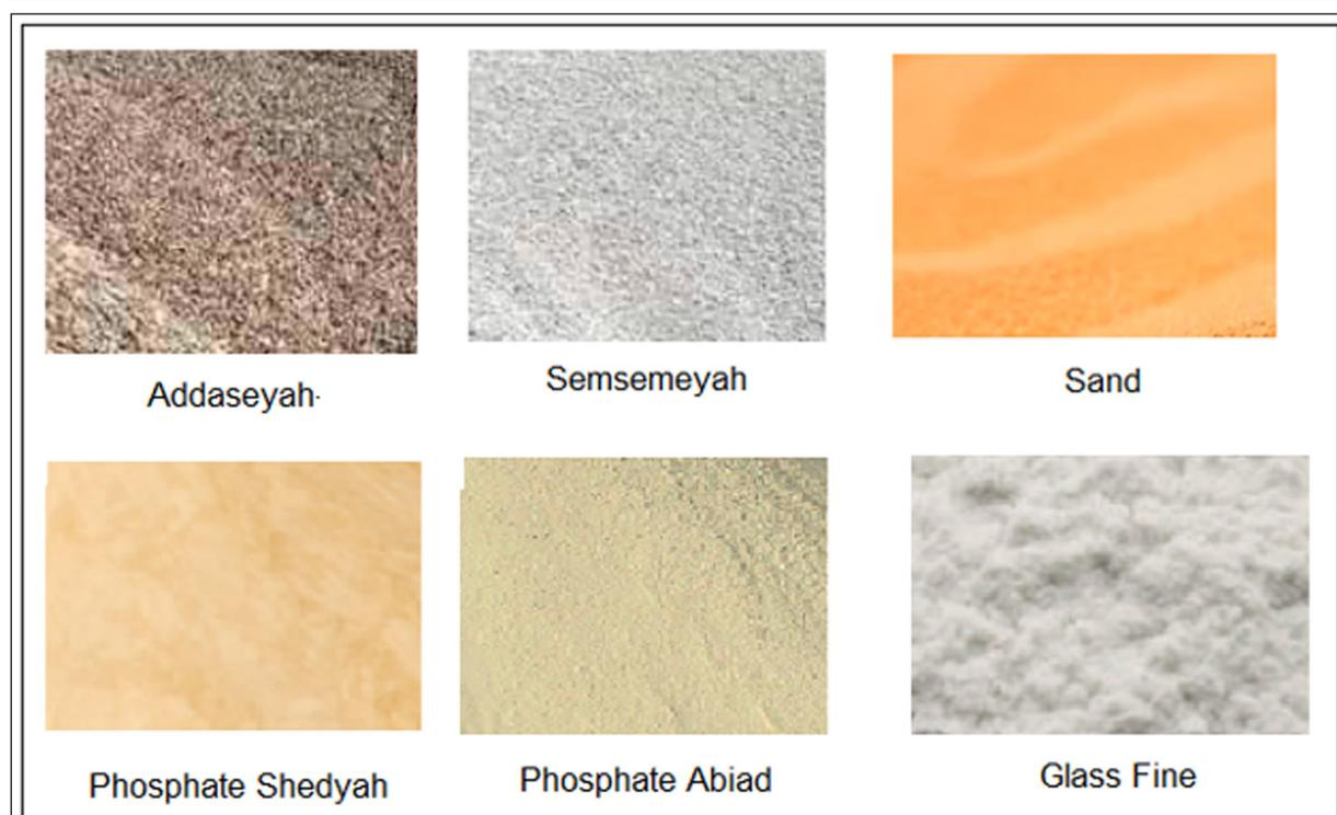
**Figure 1.** Materials of Fine Concrete Mix Design.
