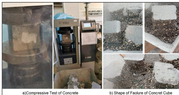
Figure 7. Compressive Strength Test and Shape of Failure for Cube Specimens.
