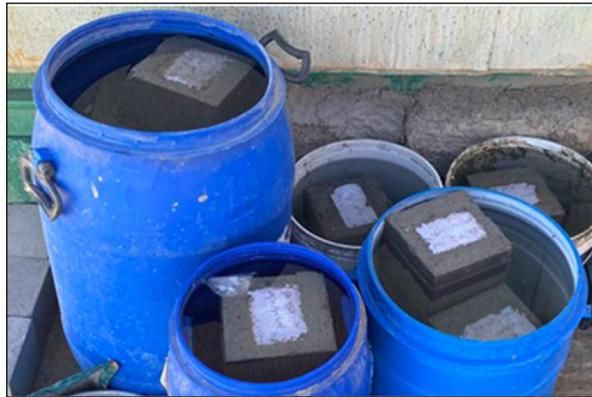
Figure 6. Curing of Concrete Samples
