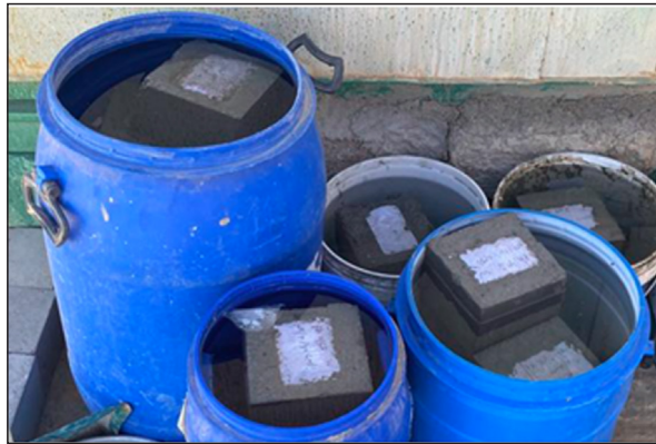
Figure 6. Curing of Concrete Samples
