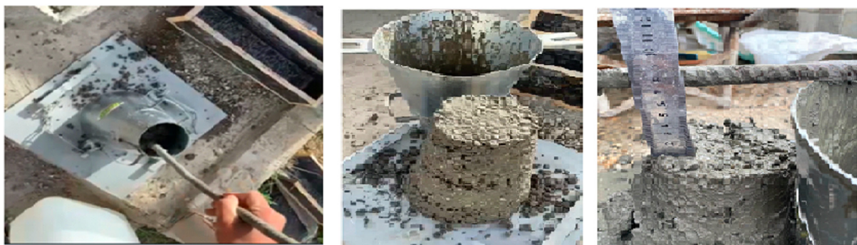
(a) Layering and Free Compaction (b) Flipping of Slump Mold (c) Measuring of Slump Value
