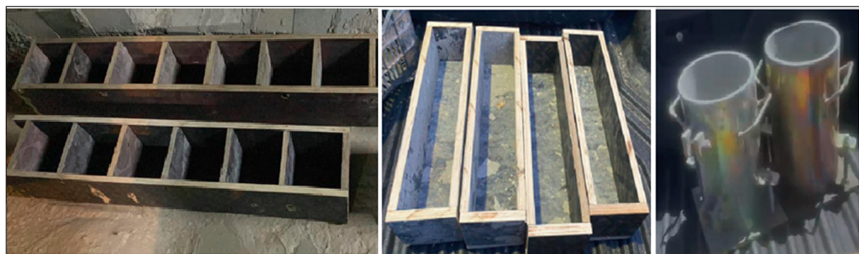
(a) Molds of Concrete Compressive Strength
