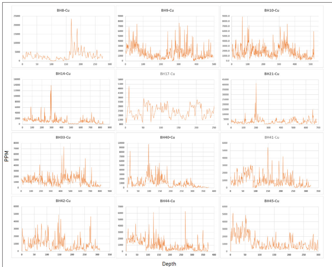
Figure 16. Cu concentration (ppm) versus depth (m) in exploratory boreholes in the study area
