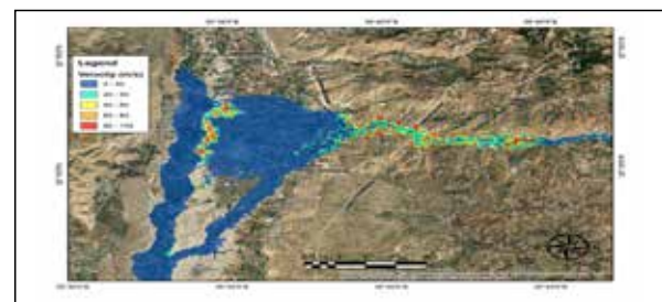
Figure 16. Velocity map due to dam failure
