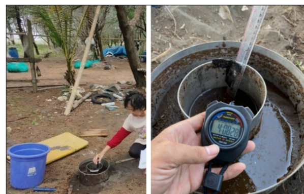
Figure 3. Example of infiltration rate measurement activity in the regosol soil zone.
