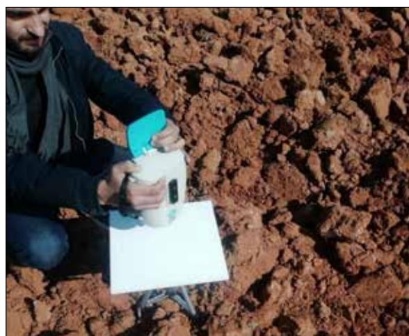
Figure 4. Calibration process of the ASD Handheld 2 Spectroradiometer using a white reference panel to ensure measurement accuracy during field data acquisition.
