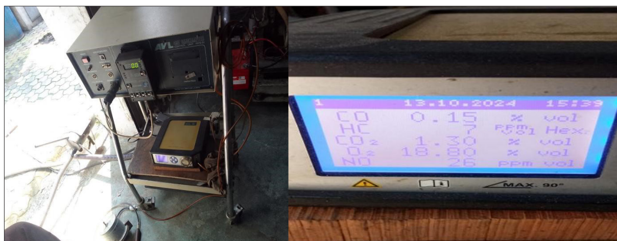
Figure 1. Smoke meter (AVL437) & Exhaust gas analyzer (AVL444N)
